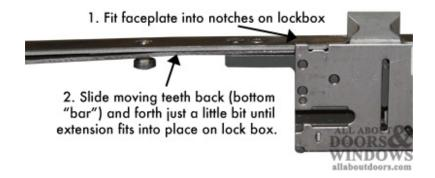
7. Hold Custom-MPL up to door edge or place in the door edge to see how hook boxes fit in mortises. You may need to lengthen mortises for both top and bottom hook boxes, though by no more than ¼ of an inch on either top or bottom of each hole. Mark with pencil where new cuts need to be made. Use razor to cut along the line. Use chisel to knock out door edge. \*\*Note: do not adjust gear box mortise—make adjustments to hook mortises only.
